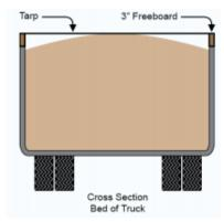
Be aware that spillage and visible emissions from a tarped load while driving on a highway constitute instances of non-compliance.
